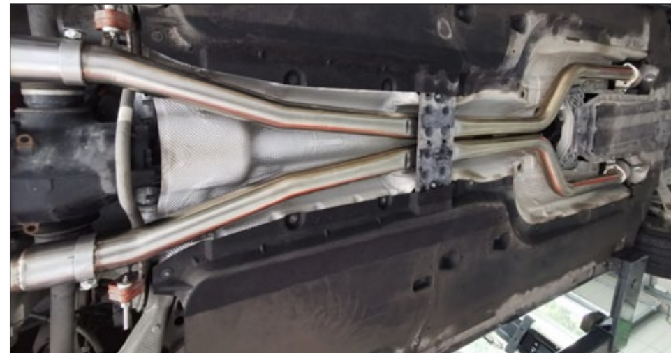
Middle pipes without muffler
