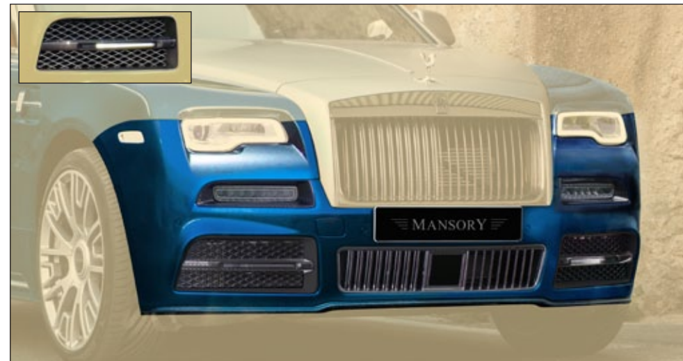
Front bumper - slim DRL for Wraith II series (MY2017) or Black Badge with LED lights RRW 102 135 with daytime running lights and fog lights front lip visible carbon fibre primed without clear coat, air intake grills primed, middle frame with slats chrom
