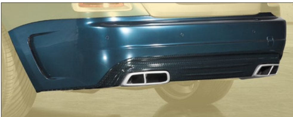
Rear bumper - chrome exhaust blinds RRW 802 031 diffuser visible carbon fibre primed without clear coat, air intakes, exhaust blinds
