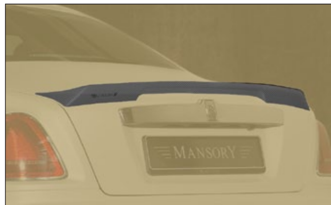
Rear decklid spoiler - exposed RR4 830 841 visible carbon fibre primed without clear coat
