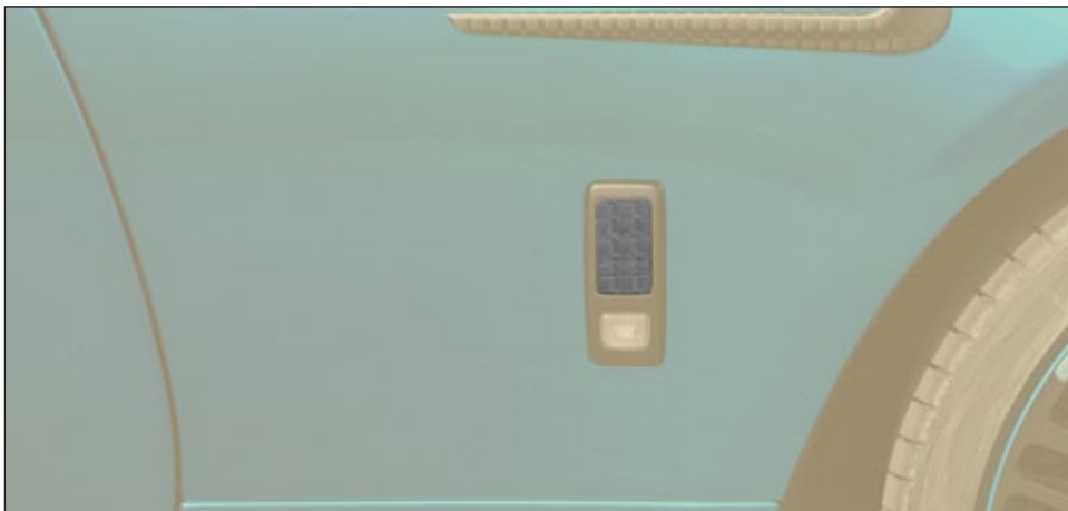
Individualized emblem for front fender with custom engraved logo RRW 130 061 visible carbon fibre primed without clear coat 2 parts set - left & right
