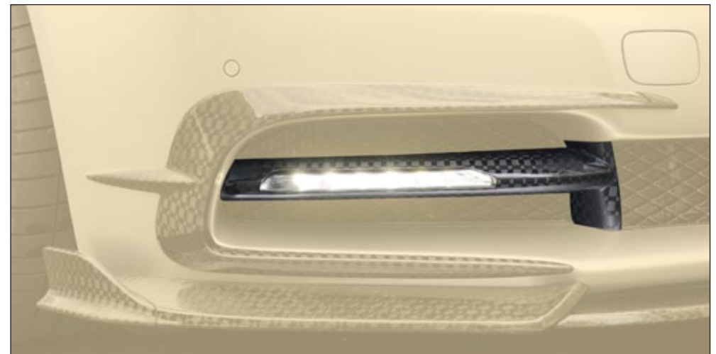
Air intakes splitter with DRL
