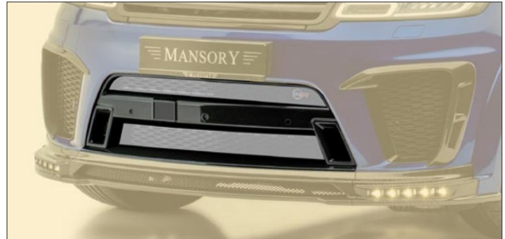
**Front bumper air intake cover - With camera**
