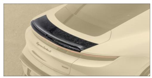
**Trunk spoiler** visible carbon fibre primed without clear coat
