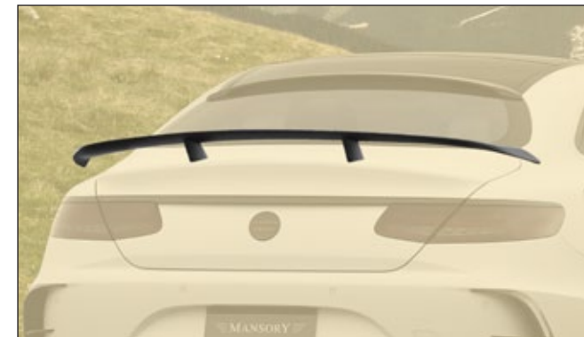
Rear dynamic performance wing ..... 217 830 341 visible carbon fibre without clear coat
