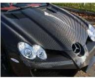
New Design Complete Engine bonnet, with visible carbon fibre
