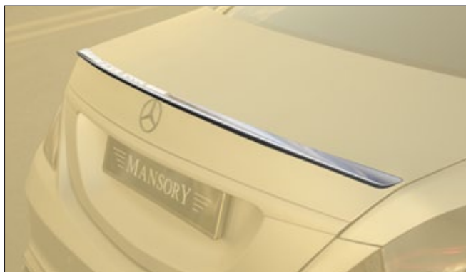
Thin rear deck lid spoiler ..... 222 830 871 visible carbon fibre primed without clear coat Thin Rear deck lid spoiler primed ..... 222 830 879 primed not visible carbon fibre
