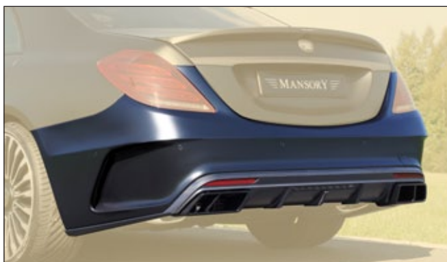
Rear bumper with diffuser visible carbon fibre without clear coat air intakes, reflectors, OEM light, exhaust blinds
