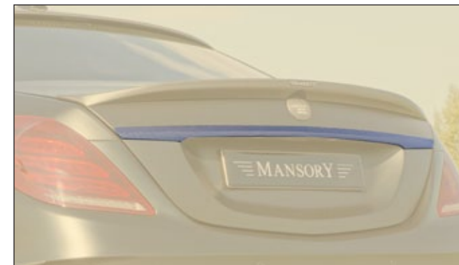
Rear bar ..... 222 802 751 visible carbon fibre primed without clear coat
