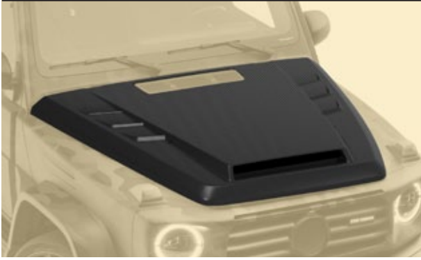
Engine bonnet I. ..... NG63 210 011 with air intake for AMG visible carbon fibre primed without clear coat
