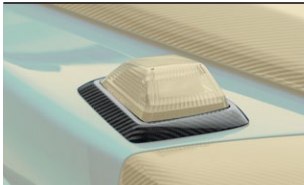
Front flasher protection cover ..... NG63 103 610 visible carbon fibre primed without clear coat 2 parts set - left & right
