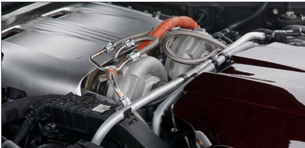
MANSORY Turbocharger upgrade C190 250 001
