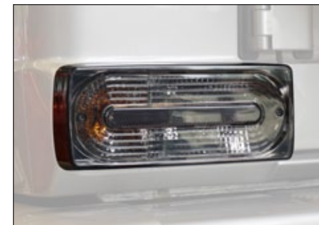
Smoky rear lights ..... 66G 804 756 to replace the original 2 parts set - left & right, including red lights for brake and tail light
