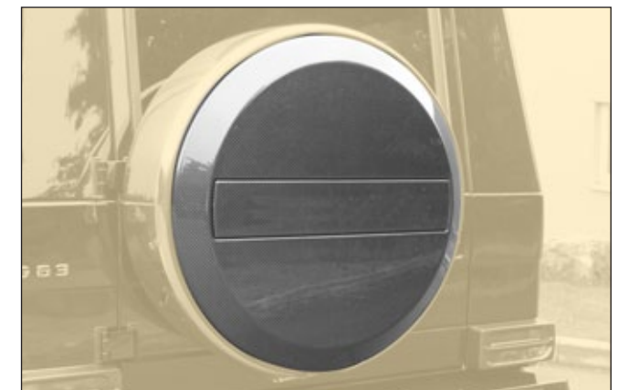
Spare wheel cover ..... G63 831 741 visible carbon fibre primed without clear coat
