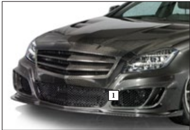
1.1 Front bumper with visible carbon lip, grill and LED DRL Ⓛ Only for car without distronic
