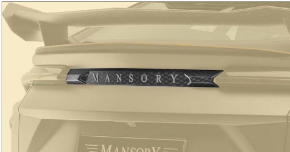
Rear hatch panel with silver MANSORY logo ..... 636 802 771 visible carbon fibre primed without clear coat
