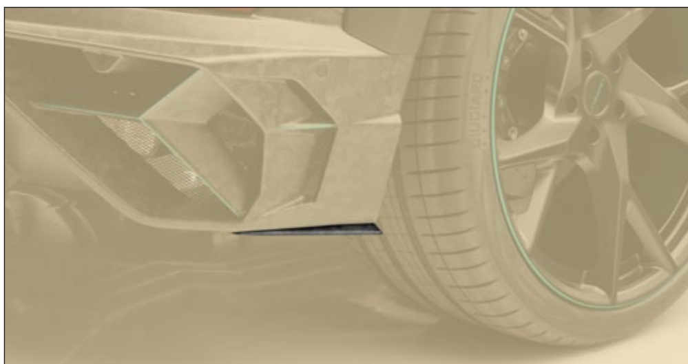
Rear diffuser extensions ..... 636 822 701 2 parts set - left & right visible carbon fibre primed without clear coat
