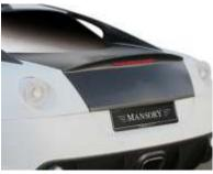
Complete Trunk Lid with Visible Carbon Fibre
