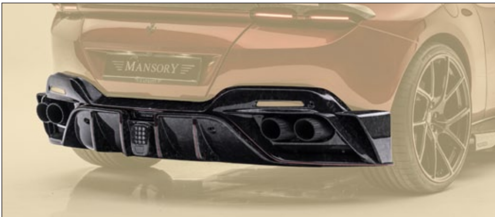
Rear diffuser with LED brake light
