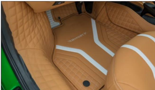
Floor mats individual FRO 367 759 with individual logo stitching, leather trim and custom colour 2 parts set - left & right
