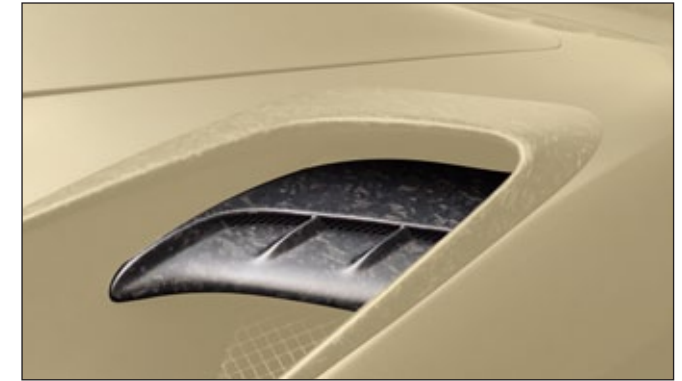
Air outtakes splitter II. ..... 488 810 561 visible carbon fibre glossy*, with logo 2 parts set - left & right
