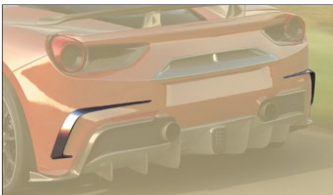
Air intake splitter 488 803 251 visible carbon fibre glossy*, with logo 2 parts set - left & right
