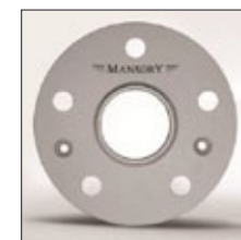
Spacer adapter kit for the widebody for CS.11 wheel BNB M11 22 FA40/RA45mm, including screws 4 parts set
