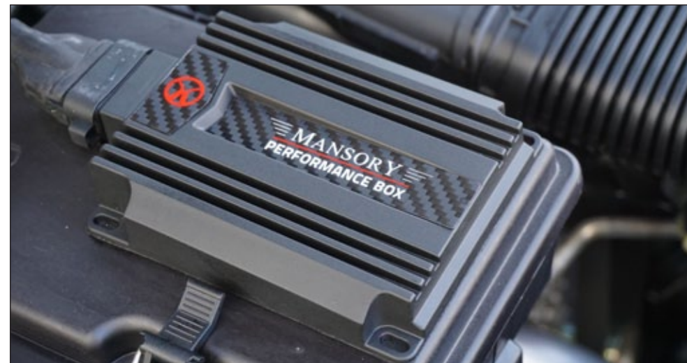
MANSORY Performance PowerBox - GT/GTC V8 ..... MPB 3S3 104 +109 PS +151NM +20KM/H MANSORY Performance PowerBox - GT/GTC W12 ..... MPB 3S3 103 +103 PS +145NM +20KM/H
