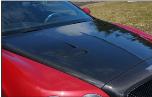
NEW engine bonnet ..... 505 110 011 visible carbon fibre without clear coat NEW engine bonnet, primed ..... 505 110 012 not visible carbon fibre
